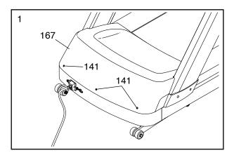
Using a handheld vacuum, clean the area under the Motor Hood (not shown). Be careful to avoid touching any components. Next, check the Drive Belt (160) for wear and cracks. If the Drive Belt needs to be replaced, see the back cover of this manual.
