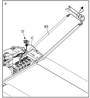
With the help of a second person, hold the handrail assembly (E) near the Left and Right Uprights (82, 83). Insert the wires (D) from the Right Upright up through the indicated hole in the handrail assembly.
