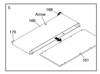
If you are replacing the Walking Platform (161), slide out the old Walking Platform and slide in the new Walking Platform.
