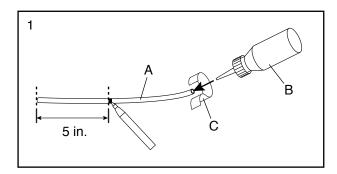
Insert the end of the tubing under the center of the Walking Belt (166). Next, squeeze the silicone bottle (B) while pulling the tubing out from under the Walking Belt until you see the mark on the tubing. Then, remove the tubing from beneath the Walking Belt. Repeat this step on the other side of the Walking Belt.
