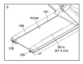
Move the Walking Belt (166), if necessary, until the seam across the Walking Belt is underneath the Walking Platform (161).
