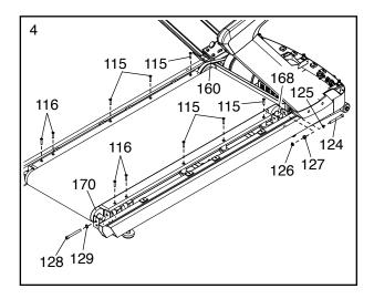
Next, remove the Drive Belt (160) from the Drive Roller (168). Then, remove the two M12 x 110mm Screws (128) and M12 Lock Washers (129) from each side of the Idler Roller (170) (only one side is shown).
